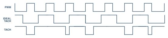
Figure 1. Tachometer-output waveforms in 3-wire fans—ideal, and under PWM control.
