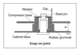
The mounting accessories for the compressors are available in two versions, with bolt joint or snap-on joint. The rubber grommets are designed for the 16 mm holes of the baseplate.
