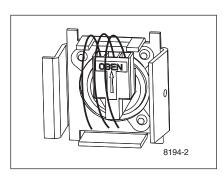
The cable plug of the electronic unit is mounted on the pins of the current lead-in on the compressor. Then the electronic unit itself is mounted on the bracket of the compressor. At first the left side is mounted, then the right side is pressed over the screw on the bracket. The electronic unit snaps on to the bracket and is now securely mounted on the compressor.
