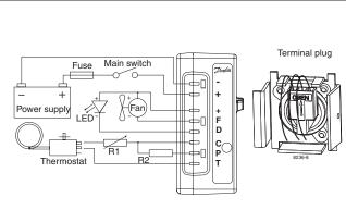
Power consumption is limited to 100W with electronic unit 101N0500.
