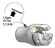
**3** Align blade (7) in hub jaw and insert pivot pin (8) with the notch in pin aligned with the hole for the tapered pivot pin locking screw (9); Move blade slightly to ease operation;
