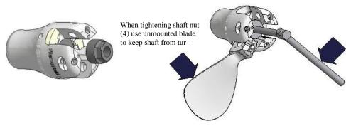
2 Mount shaft nut locking screw (5) using the Allen wrench (13) supplied. If using torque wrench tighten to about 1 Kpm=10 Nm=7.2 ft-lb;
