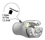
**3** Align blade (7) in hub jaw and insert pivot pin (8) with the notch in pin aligned with the hole for the tapered pivot pin locking screw (9); Move blade slightly to ease operation;
