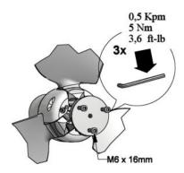
**6** Mount sacrificial anode (11) Zn or AlMg, with one socket-head cap screw (12) after having applied thread locker to threads if not already applied. Again work blades open and folded to ensure ease of operation;
