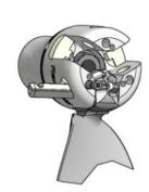
4 Continue with the next two blades; Work blades open and folded to ensure ease of operation; Tighten all pivot pin locking screws using the Allen wrench supplied. If using torque wrench tighten to about 1.2 Kpm = 12 Nm = 8.4 ft-lb.; Again work blades open and folded to ensure ease of operation;
