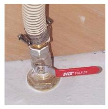
Thru-hull fitting closed
