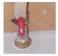
Thru-hull fitting open
