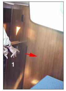
1. Remove the port engine hatch.
