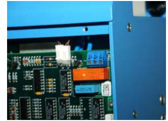
The connection for the Virtual Switch is located at the top-right of the controller PCB.
