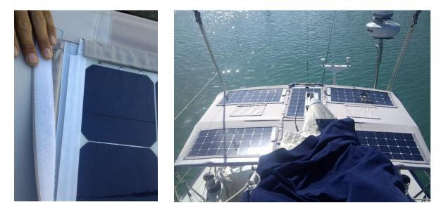
Note that the Velcro is both sewn and glued to the panel. Also note that in this case a bit more clearance could have been left between the Velcro and the cells to avoid shading the cells.
