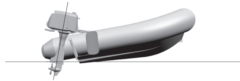
Bow up, too much trim-out
