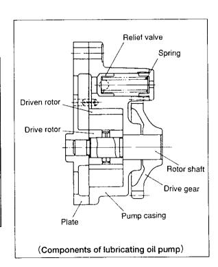
②Disassembling the lubricating oil pump
