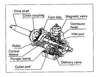
b) There are two plunger springs having setting forces on the outside of the plunger. They return the plunger which is pushed up by the cam disc, in the descending process. That is, the plunger rotates by means of the drive shaft and reciprocates by means of the cam disc. When the fuel whose pressure is increased by the plunger is sent to the outlet port, the delivery valve opens to allow the fuel to be injected into the combustion chamber through the fuel injection nozzle.
