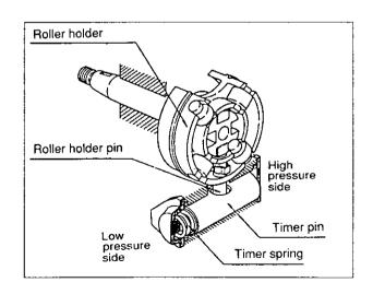
in the reverse direction of rotation) to advance the injection timing. That is, the timer controls the injection timing according to the fuel oil pressure in the pump house.
