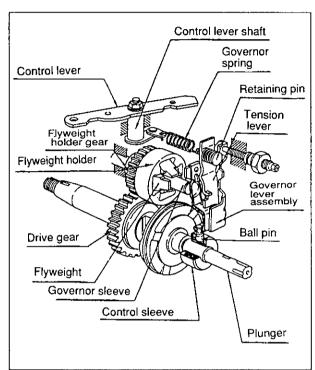
The control lever is linked to the governor handle through the link to vary the setting force of the governor spring according to the inclined angle. A difference between the setting force of the governor spring and the centrifugal force of the flyweight corresponds to the control sleeve movement which increases or decreases the injection quantity.
