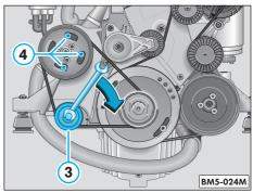
• Insert the seawater pump in the bracket and secure it with the screws **4** on the bracket.
