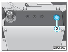
• Press and hold the button **2** on the fuse box/relay plate with the ignition switched on until the motor oil is completely pumped out.
