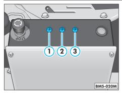
The individual circuits are protected with fusible links.
