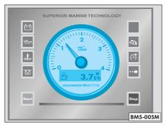
The illustration shows the rev. counter of the flying bridge panel.
