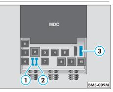
The fuses are located in the fuse box/relay plate behind the cover.
