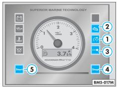
The illustration shows the switches of the flying bridge panel.
