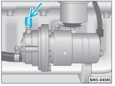
• Remove the cover of the oil filter so that the return valve opens and the used oil can flow back into the oil sump.
