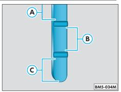
Then pull out the oil dipstick again and read off the oil level:
