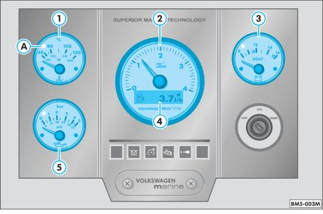
The illustration shows the instruments of 1 - Coolant temperature the navigating stand panel.
