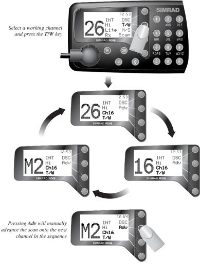
Note As with Dual Watch, normal VHF functions will not be available when in Tri-Watch mode. Exit Tri-Watch by pressing 16 or C.
