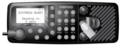
To send the call, **press and hold** the **DISTRESS** key for five seconds. A countdown to the transmission will be displayed. Release the key at any time during this countdown to abort the transmission and press C to return to the main menu.
