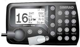
There are five levels of brightness – press and hold the \* key to step through and release when the required level is shown.
