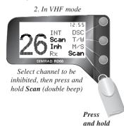
To re-enable an inhibited channel into the scan cycle, repeat sequence 2:
