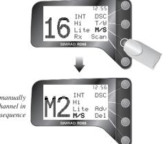
Press Adv to manually advance to the next channel in the Memory Scan sequence
