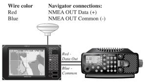
Fig 4.5 - Linking to navigation source
