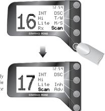
Press Adv to manually advance to the next channel in the scan sequence
