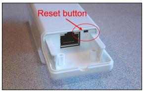
button depressed varies from 10 to 20 seconds. Caution: If you see an alternating two LED pattern that goes back and forth, turn the power off for 5 seconds and start the procedure again.
